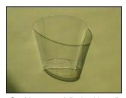
Cracking, especially in thin-wall parts, can result from orientation due to overly rapid injection. Try varying the injection speed or, if possible, moving the gate.
