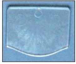
Ripples or "record grooves" are a common defect, which signify hesitation of the flow front owing to inadequate injection pressure or slowing injection velocity.
