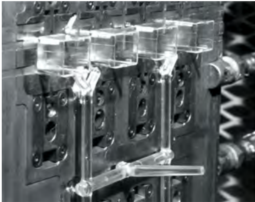
The injection molding process can quickly produce large quantities of parts in multi-cavity molds.
