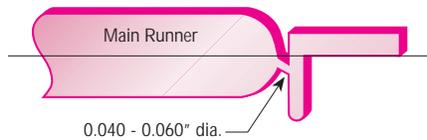
**Pinpoint or Restricted Gate** - A restricted opening between the runner and molded part. Normally used with thin wall parts.
