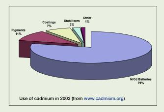
Cadmium sulphide and cadmium sulphoselenide are utilised as bright yellow to deep red pigments in plastics, ceramics, glasses, enamels and artists colours. They are well known for their ability to withstand high temperature and high pressure.
