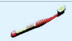
This toothbrush has been co-injection moulded. Two incompatible materials that cannot be recycled together are now permanently bonded, making disassembly nearly impossible. The designer might have considered using different coloured components that could slot together, or using different colours of the same material (from: Sustainable Design Awards <a href="https://www.sda-uk.org">www.sda-uk.org</a>).
