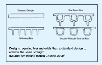
In some cases, for example, it may be possible to increase plastic stiffness by using engineering techniques, instead of increasing the amount of plastic used. Examples of these techniques are shown above.
