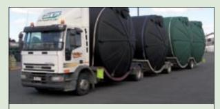
RX Plastics had the deck of a truck completely modified to be able to handle the transportation of their water tanks. They have maximised loading potential and ensured their product gets delivered safely and securely.
