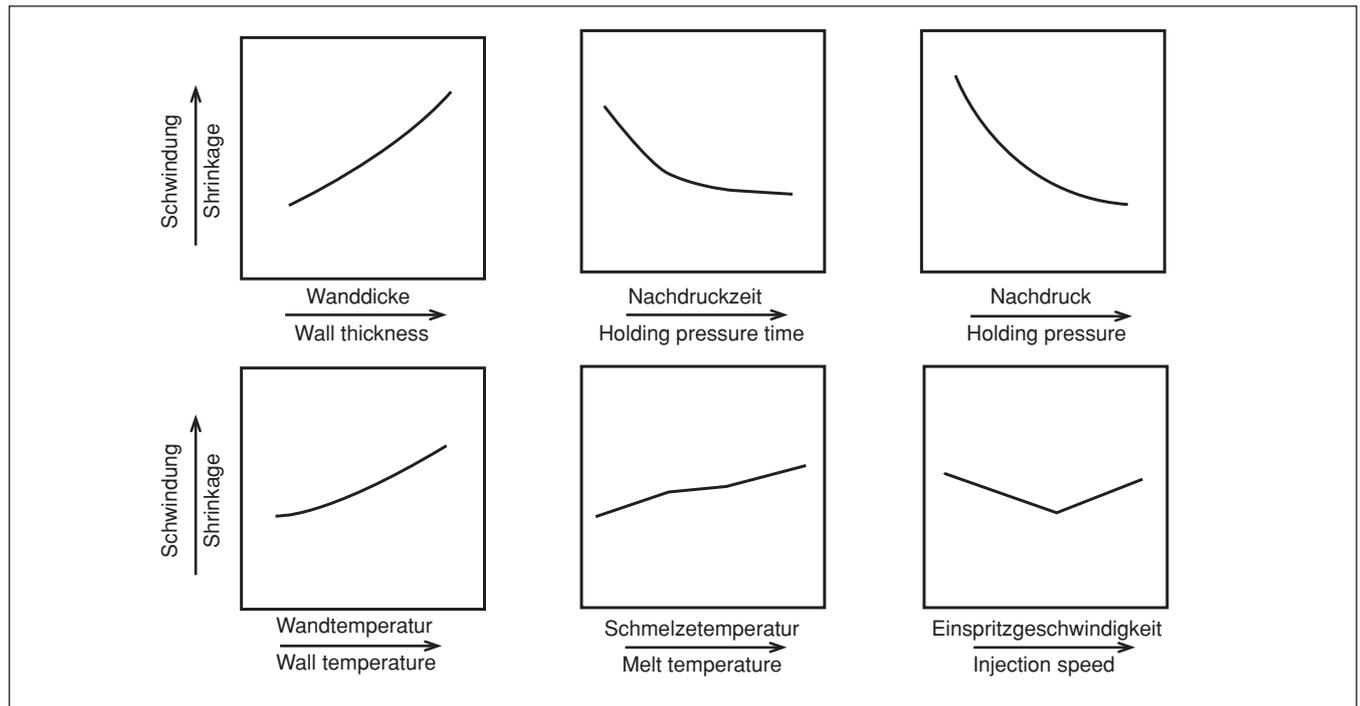
Fig. 2: Qualitative relations between individual process parameters and shrinkage behavior
