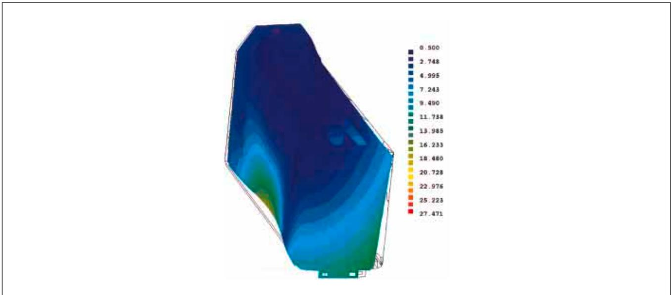
Fig. 8: Deformation of a molded part in its actual condition, computed according to Autodesk-Moldflow
