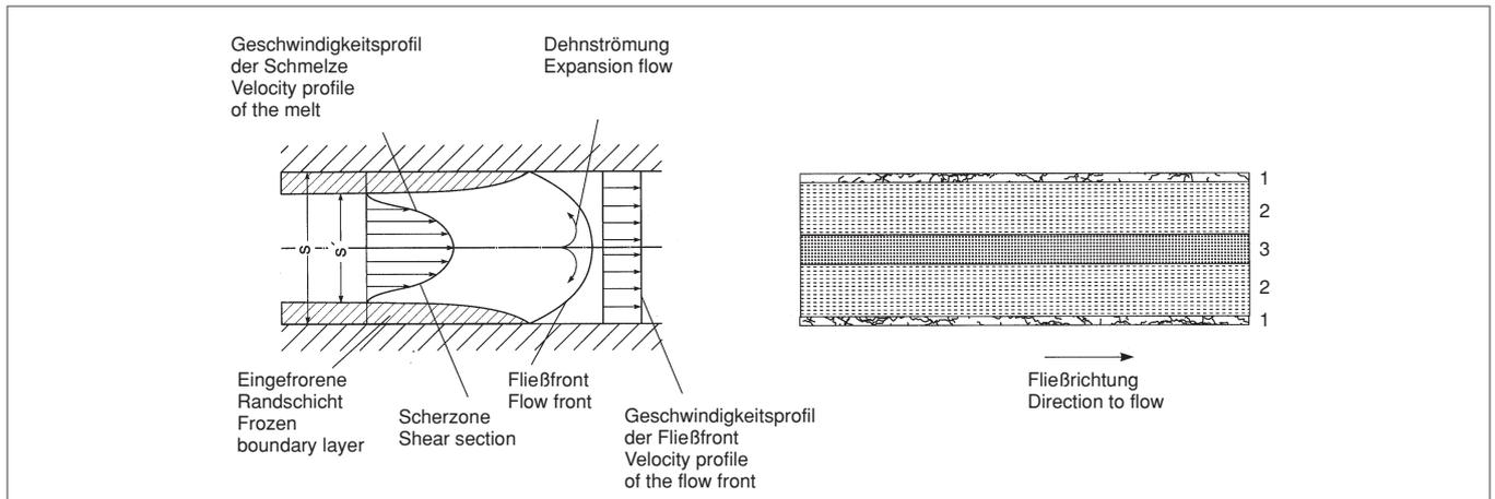
Fig. 4: Flow conditions in a thermoplastic melt (left) and different orientation zones over the flow cross-section (right) [2]
