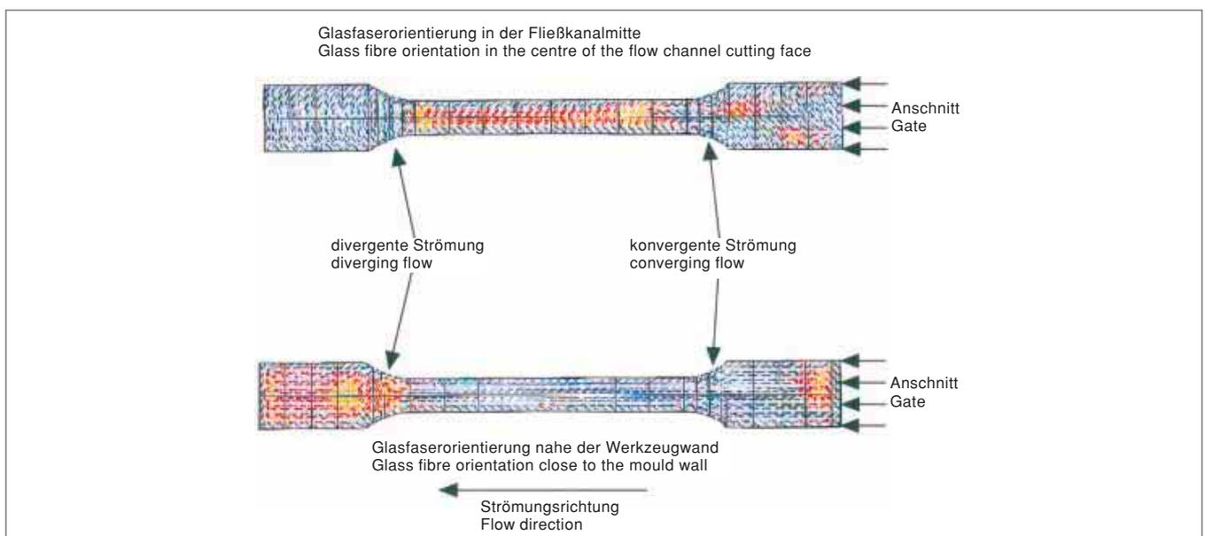
Fig. 5: Glass fiber orientation in a tensile bar (program: Autodesk-Moldflow)
