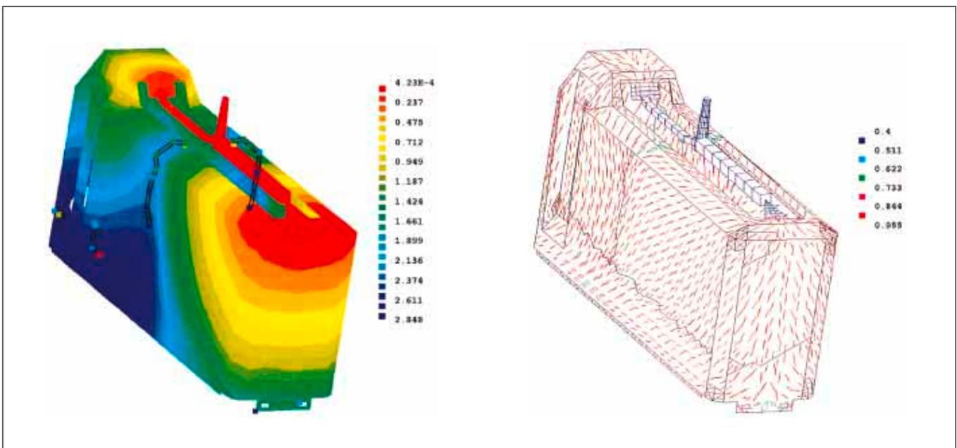
Fig. 7: Computed filling of the molded part (left) and respective glass fiber distribution in the shear zone (right) computed according to Autodesk-Moldflow
