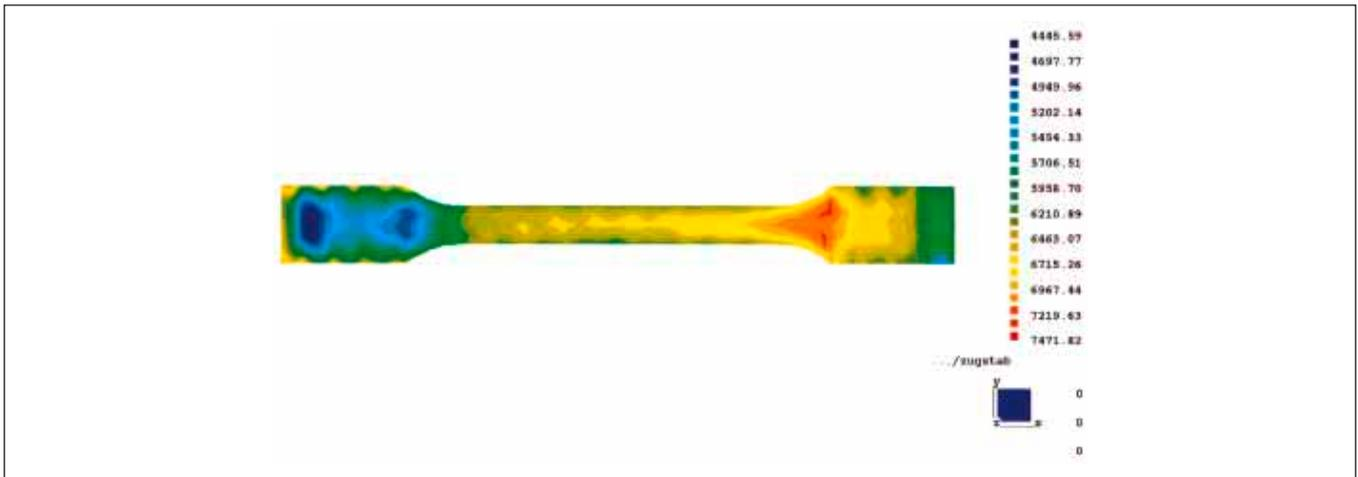
Fig. 6: Distribution of the elasticity modulus parallel to the flow direction, calculated according to the Ogorkiewicz-Weidmann-Counto material law (program: Autodesk-Moldflow)
