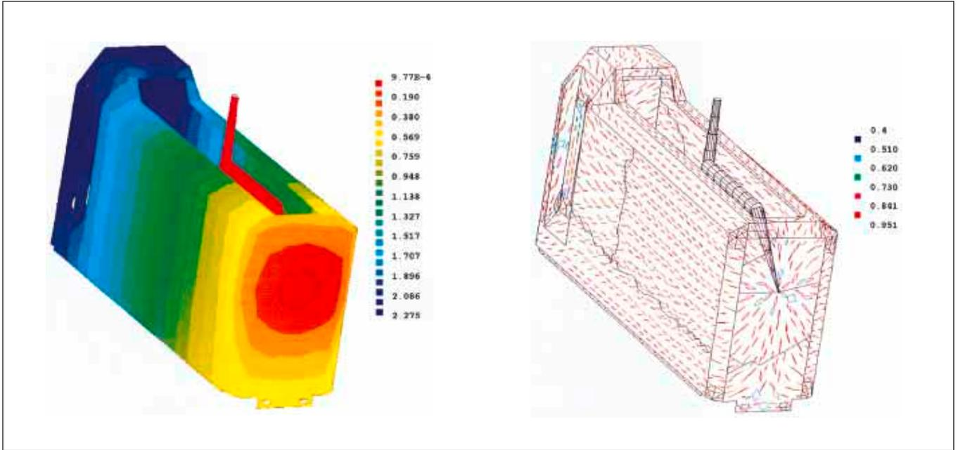
Fig. 10: Filling of the molded article (left) and glass fiber orientation (right) after mold change, computed according to Autodesk-Moldflow
