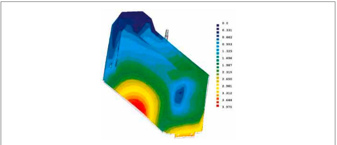
Fig. 11: Calculated deformation after mold changes computed according to Autodesk-Moldflow
