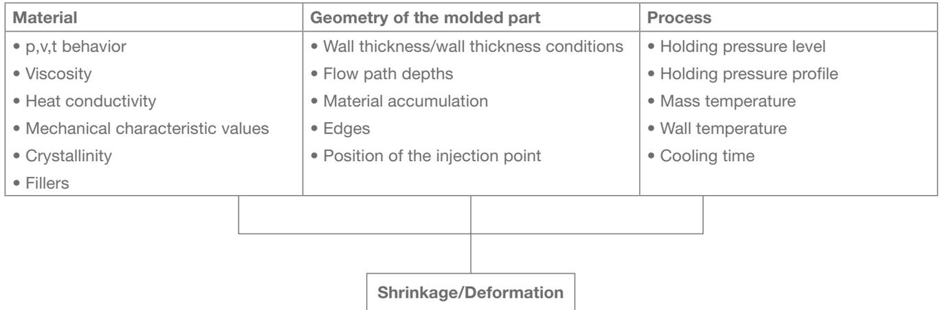
Fig. 1: Factors affecting the shrinkage and deformation of thermoplastic injection molded parts [1]
