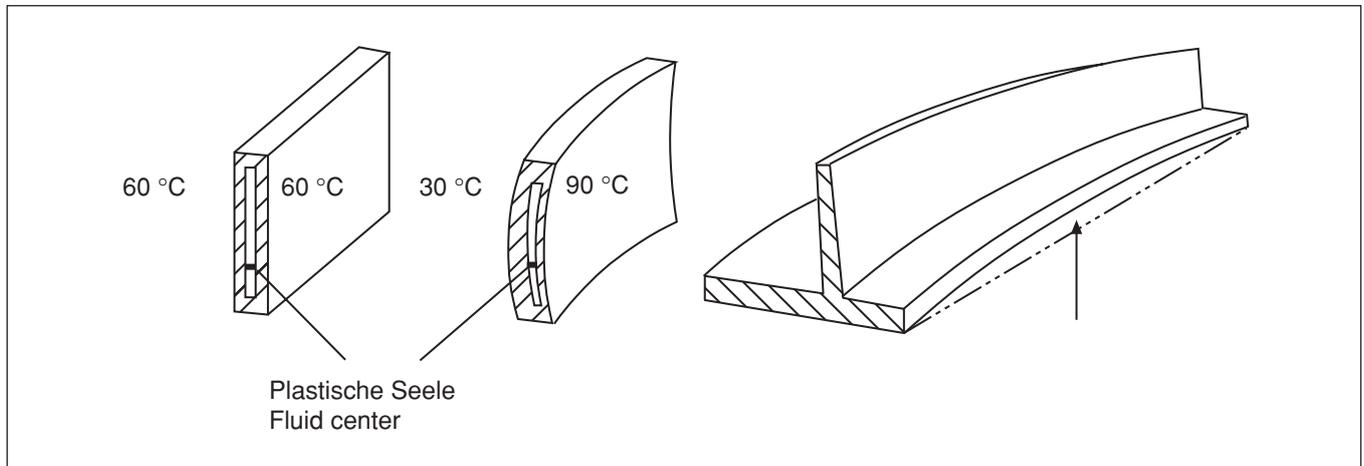
Fig. 3: Deformation of a sheet as a result of differences in the wall temperature (left) and the presence of a rib with a lesser wall thickness (right)
