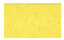
Specks can be due to contamination of the polymer or to resin degrading in a dead spot in the screw flights and being carried through with the next shot. Streaks derive from contamination on the screw, such as degraded material in a dead spot, or from the wrong screw design. Poor color mixing can be due to the screw design or incompatibility between the substrate and the colorant.
