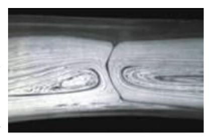
or it can significantly weaken the structural integrity of a part. Strength at the knit line can be as little as 20% of the nominal strength of the part—or it can be 100% as strong, depending on a host of variables.
