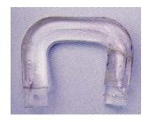
**Black streaks** caused by introduction of air into the feed and subsequent carbonization when the polymer is injected into mould.
