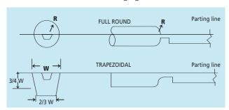
The round runner terminates in a spherical shape which traps cool material at the outside while passing hot material at the center of the runner.
