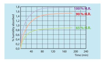
To eliminate the need or waiting for humidity, the parts may be cooled to service temperature in a dedicated atmosphere and a correction factor added to the part size based on the humidity conditions the parts will encounter in service.
