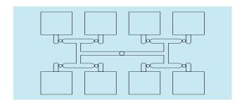
The balanced runner system requires slightly more material for each shot than an unbalanced runner system but this is off set by improved yields of good parts. This system can be used to fill 4-8-16-32 cavities only.
