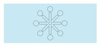
As with the balanced H runner layout the spoke runner layout uses the same runner length from the sprue to each cavity.
