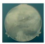
Post annealing & ethanol testing: residual stress: NO, orientation stress: YES
