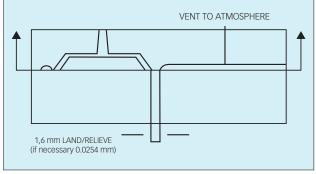
The continuous venting technique ensures adequate venting and since it is incorporated into the initial design of the mould; continuous venting may cut the time required to put the mould into production.
