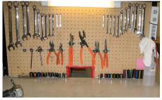
Sockets are color coded to make sure the correct tool is used according to the work instructions.
