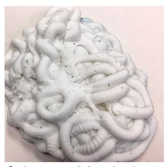
Examine your purge pile for specks and uneven color distribution. If there are random specks in the pile as shown here, then your streaks are likely being caused by the screw and barrel.
